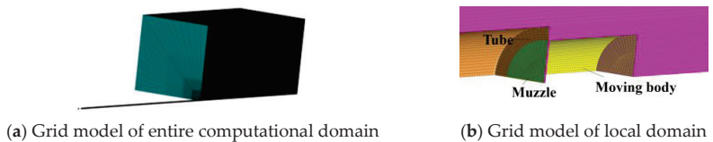
Figure 2. Schematic diagram of grid model of the muzzle jet of a large-caliber long-barrel launcher.
