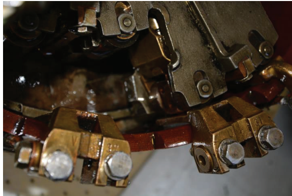
Figure 2. Modified OLTC contacts.
