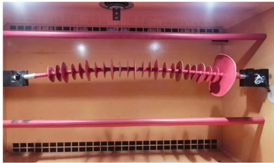
Figure 6. Schematic diagram of the composite insulator bearing a bending load.
