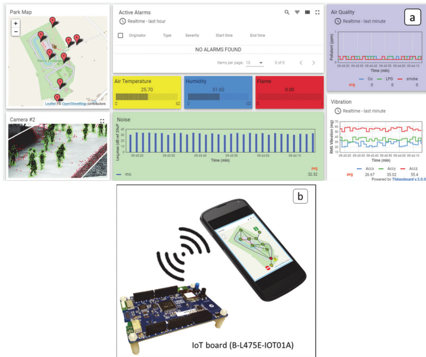
Figure 5. (a) IoT system dashboard; (b) Emergency plan provided by the NFC module-smartphone connection in the form of a smartphone compatible map.
