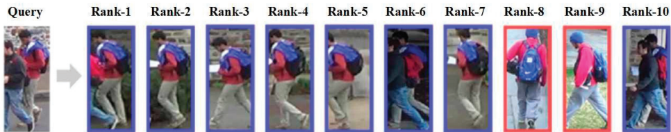
Figure 7. One example query image in DukeMTMC-reID dataset and ranking list results from Rank-1 to Rank-10 using MFF model. The blue boundary means true positive and red means false positive.
