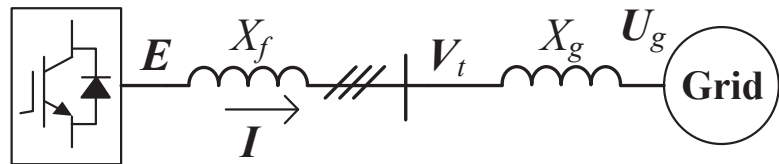
Figure 8. Simplified network topology.
