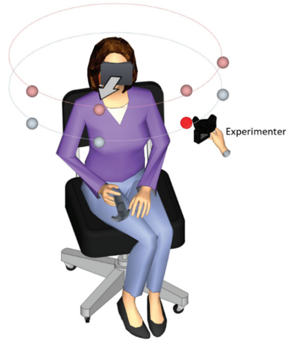
Figure 2. Experimental setup of head-pointing localization task (LOCATEST). The illustration shows the participant wearing the head-mounted display (HMD) during the LOCATEST. The eight spheres indicate predetermined speaker positions, which were not visible in the HMD. The hand holding the speaker near the red sphere was the experimenter's hand, who moved the speaker to reach the target position.
