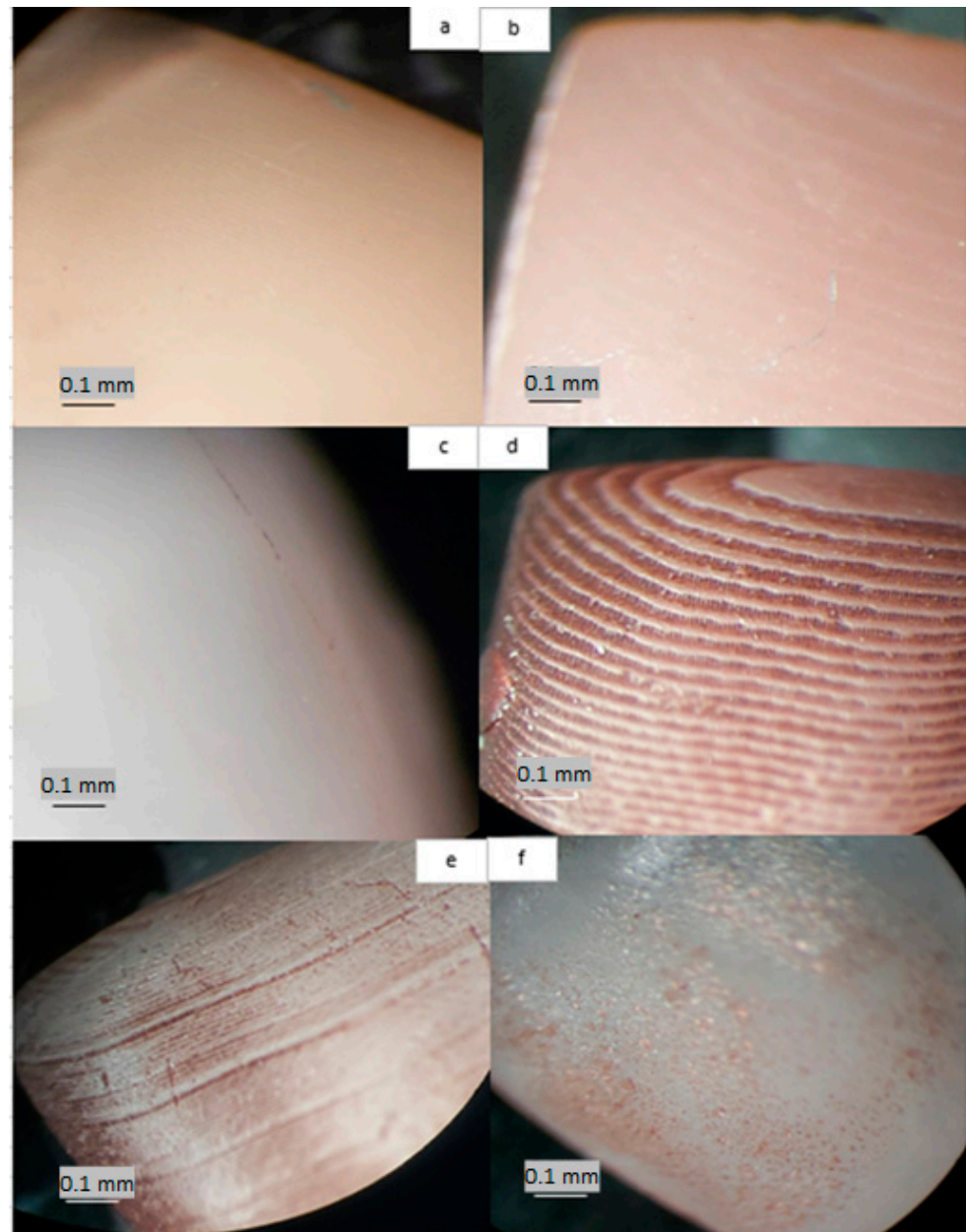
Figure 4. (a) Photograph of the tooth surface under a microscope. It is visible that polishing the tooth surface provides less retention for dyes (Crowntech A3); (b). Teeth covered with varnish are protected against discoloration, but after a long time, the protecting layer can crack (Crowntech A2); (c) Teeth covered with varnish, after storage in distilled water. Lacquer cracks (arrows), and the remnants of dyes begin to accumulate in the gaps (Crowntech A2). (d) Teeth’s unpolished surface after storage in red wine, and (e) after contact with coffee. Between the individual layers of the material as it was printed are visible dyes (Crowntech A2). (f) Sample of A2 color storage in red wine for 60 days, with a polished surface but not enough; a clearly visible region with greater roughness, where the absorption of dyes took place (Magnification 25×).
