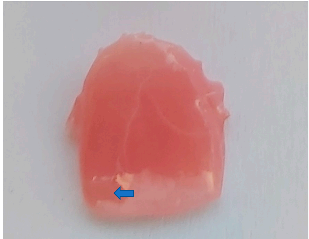
Figure 2. Deture base material Denture 3D +. The surface of the sample is covered with varnish and stored in distilled water. Under the influence of storage, the varnish separates from the resin. Separation is marked with arrows.
