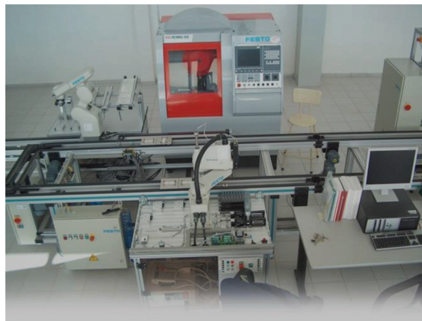
Figure 7. Traditional CPS: iCIM3000 didactic cubicle.
