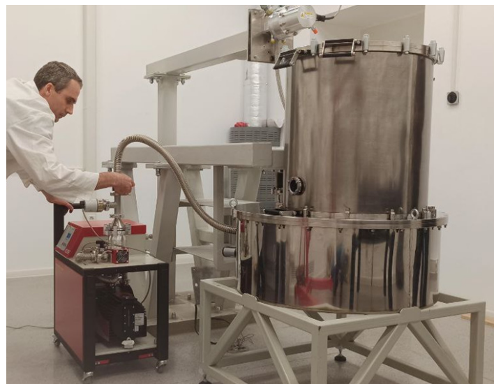
Figure 23. Photo of the 4 K cryosystem for studying thermal deformations of the mirror panels of the Millimetron space mission installed in P.N. Lebedev Physical Institute RAS, June 2023.
