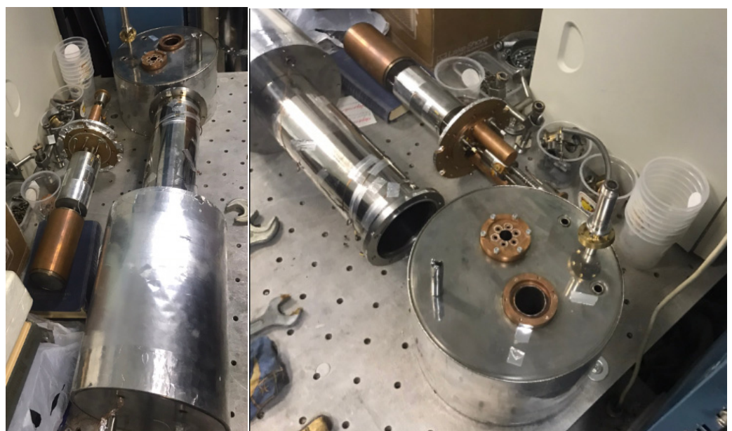
Figure 7. The 0.3 K sorption cryostat.
