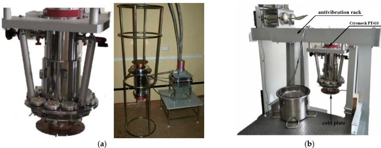
Figure 12. Photos of the 4 K cryostating system based on a pulse tube: (a) general view; (b) the cryosystem mounted on an antivibration rack in order to increase the accuracy of measurements.
