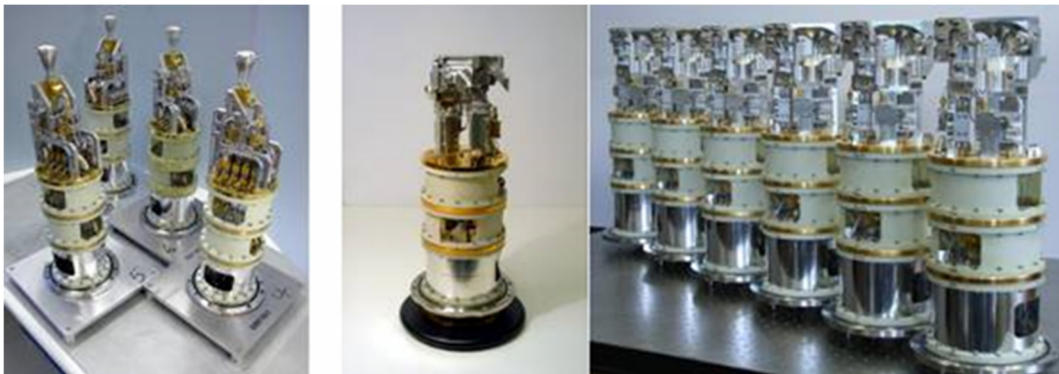
Figure 5. Cryogenic cartridges of ALMA receivers.
