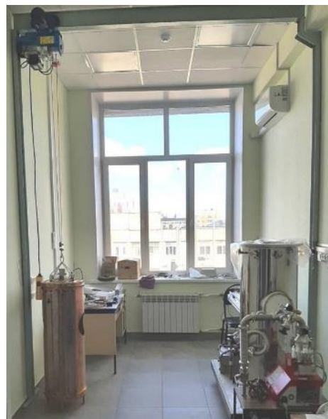
Figure 26. A new vacuum stand for the study of gas spectra in the subTHz frequency range at temperatures from -50\text{ }^{\circ}\text{C} to +200\text{ }^{\circ}\text{C} , IAP RAS, May 2023; “the first launch” in November, 2023.
