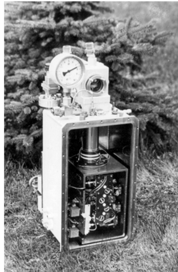
Figure 6. Photo of the 20 K cryogenic radiometer of 4 mm band.
