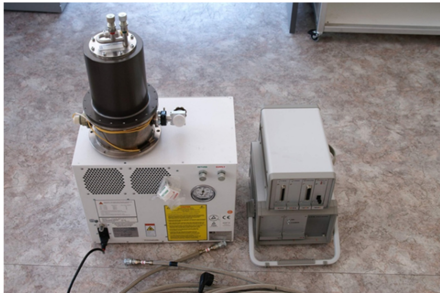
Figure 3. Optical cryostat based on the CryoTiger refrigerator.
