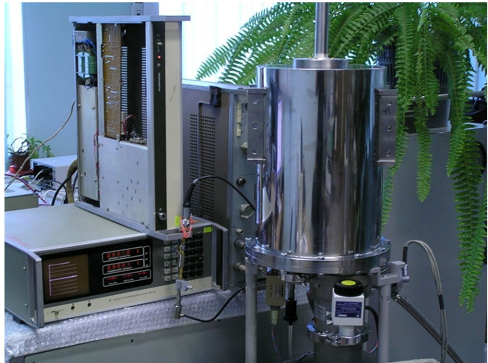
Figure 4. Cryogenic system for cooling of the X-band receiver.
