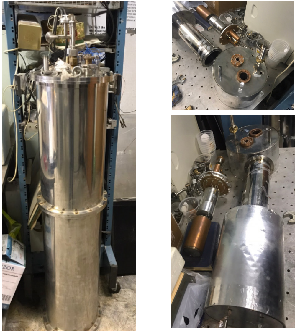
Figure 9. The 0.3 K sorption cryostat.
