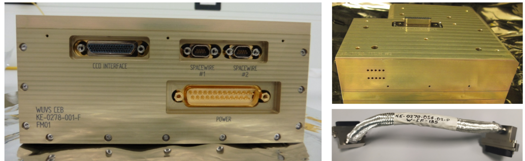
Figure 6. Flight models of the camera electronic box (CEB), interconnection module (ICM) and analog video cable.
