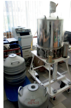
1—nitrogen tank, 2—main frame, 3—upper part of the cryostat body, 4—lower part of the cryostat body
