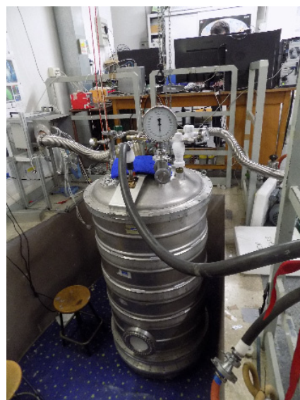
Figure 10. Cryostat for the OLYMPO balloon mission.
