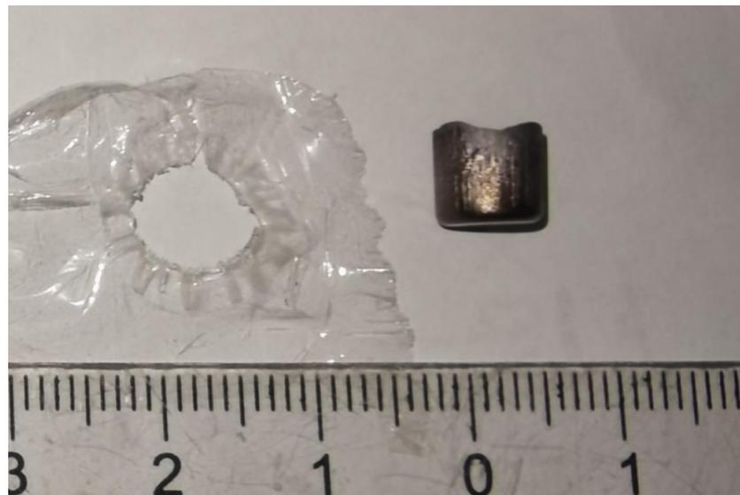
**Figure 4.** Deep drawing under the PE film.
