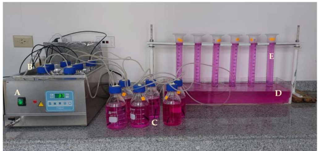
Figure 1. The experimental facility used in the research. (A) Thermostated water-bath with recirculation. (B) Anaerobic digester flasks. (C) Bubbling traps for CO 2 capture. (D) Immersion cuvette. (E) Inverted test tubes for methane measurement.
