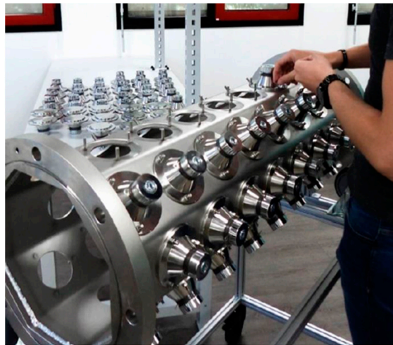
Figure 8. Installation of the transducers at Cedrat Technologies.
