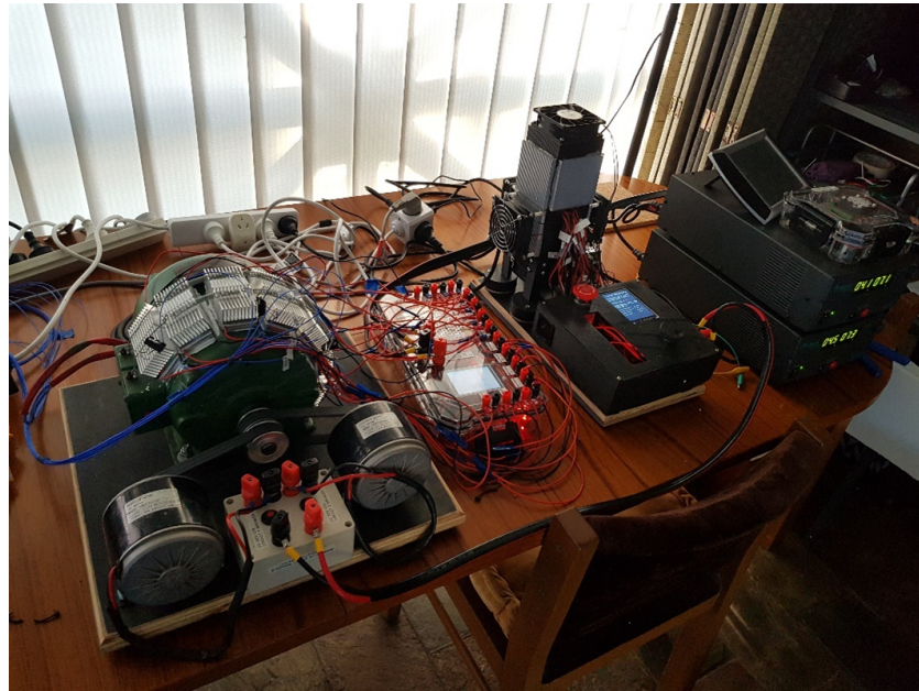
Figure 9. The setup of the heating of the test motor with the TECs and small heat sinks.
