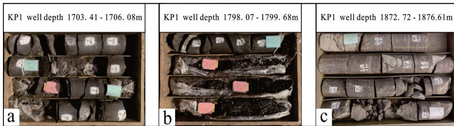
Figure 2. Core lithology maps of the Taiyuan Formation and Shanxi Formation of Well KP1 in the study area. (a) The dark-grey fine sandstone of the Shanxi Formation is interbedded with a thin layer of dark-grey sandy mudstone. (b) Grey-black sandy mudstone of the Taiyuan Formation. (c) The interbedded deep grey siltstone, fine sandstone, and grey-black sandy mudstone of the Taiyuan Formation.
