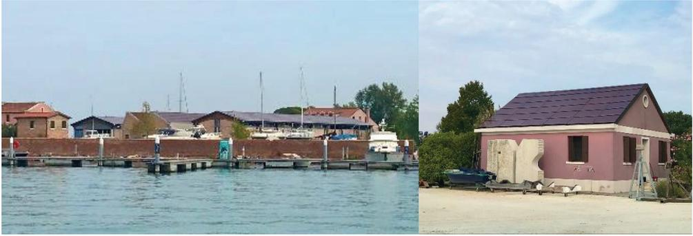
**Figure 6.** Positive example of the “*minimum intervention*” criteria on the PV roof of the La Certosa Island in Venice (Italy) with respect to the geometries, shapes, proportions, colors, and reflectance of traditional clay roofs [74] (Source: Elena Lucchi).
