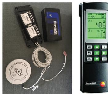
**Figure 2.** ThermoZig datalogger (left) and Testo 645 digital humidity/temperature measurement device (right).
