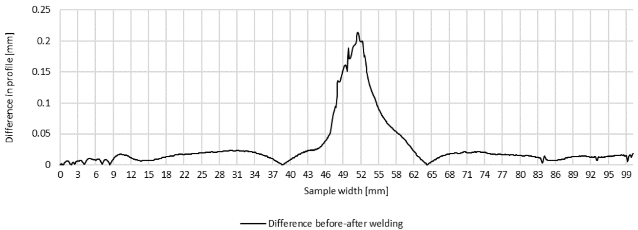
Figure 5. Difference in transverse profiles on line A before and after manual welding.
