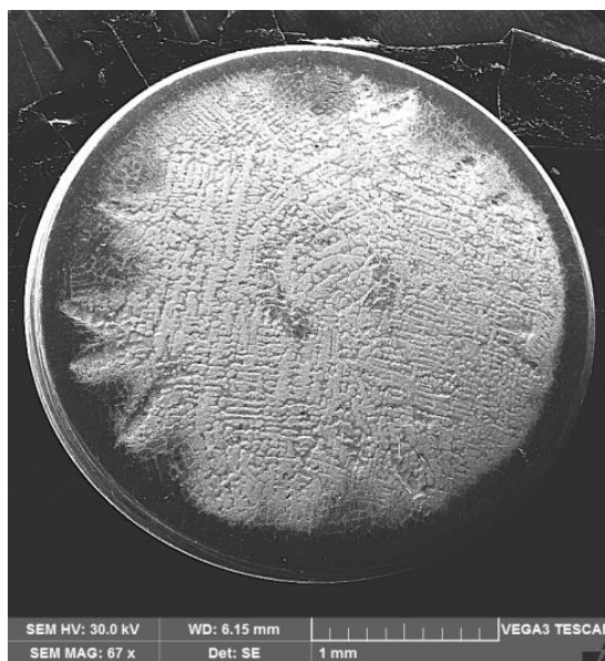
Figure 11. SEM macrograph of the unmelted surface tested by cavitation after 165 min.
