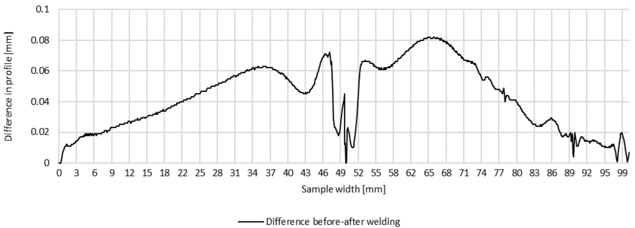
Figure 6. Difference in transverse profiles on line B before and after manual welding.
