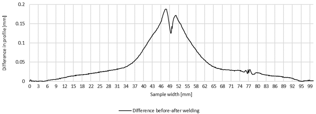
Figure 9. Difference in transverse profiles on line B before and after automated welding.
