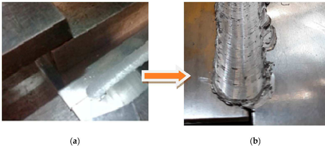
Figure 17. End areas of the joint. (a) heterogeneous joining obtained with FSW process. (b) flashing at the end of the joining.
