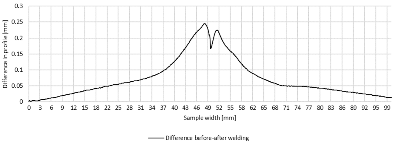
Figure 10. Difference in transverse profiles on line C before and after automated welding.
