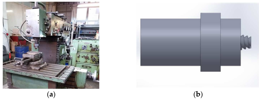
Figure 3. Equipment used for the FSW experiments, consisting of a mill machine with the following characteristics: Speed control (a); FSW tool manufactured for the present work—the length of the pin: 2.62 mm (b).
