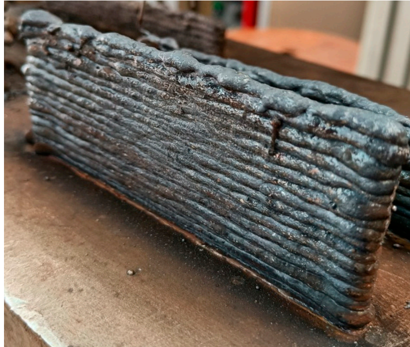
Figure 9. Multi-layer structure at optimal parametric settings.
