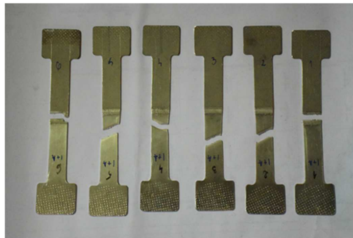
Figure 8. Pictures of the six specimens after the tensile test.
