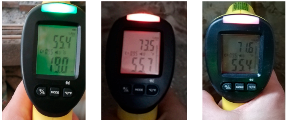
Figure 1. Examples of air humidity and air temperature tests using a pyrometer and a dew point scanner.
