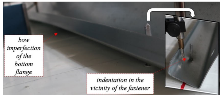
Figure 9. Failures in the nonlinear stage of the kinematical response of the connection (stage II) using self-drilling fasteners (F).
