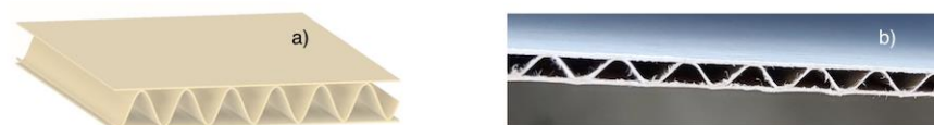
Figure 1. Structure (a) and cross-section (b) of corrugated cardboard sample used for this study.
