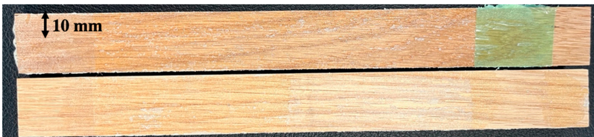
Figure 16. DCB specimens' fracture surfaces.
