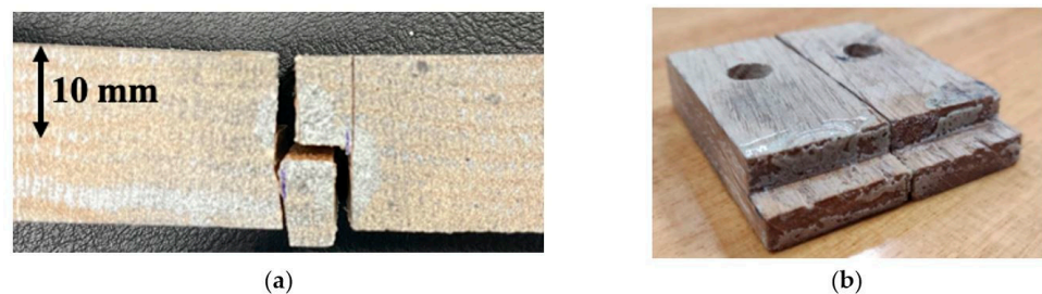
Figure 14. Fracture surface of TAST specimen: substrate loaded in transverse direction (a); substrate loaded in fiber direction (b).
