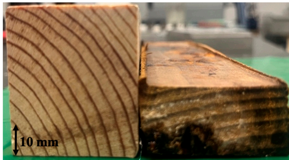
Figure 9. Wood beam before (left) and after (right) densification.
