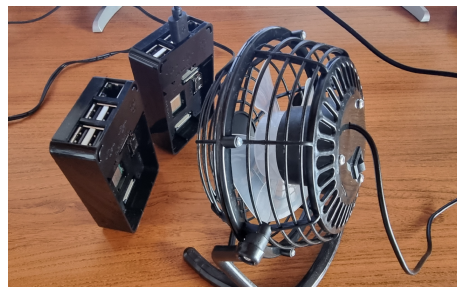
Figure 2. Cooling Mechanism for Raspberry Pi Devices.
