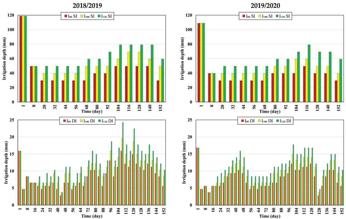
Figure 2. Applied irrigation water at the timing intervals for different treatments in both growing seasons. I_{80} = 80% crop evapotranspiration ( ET_c ), I_{100} = 100% ET_c , I_{120} = 120% ET_c , SI = surface irrigation, and DI = drip irrigation.
