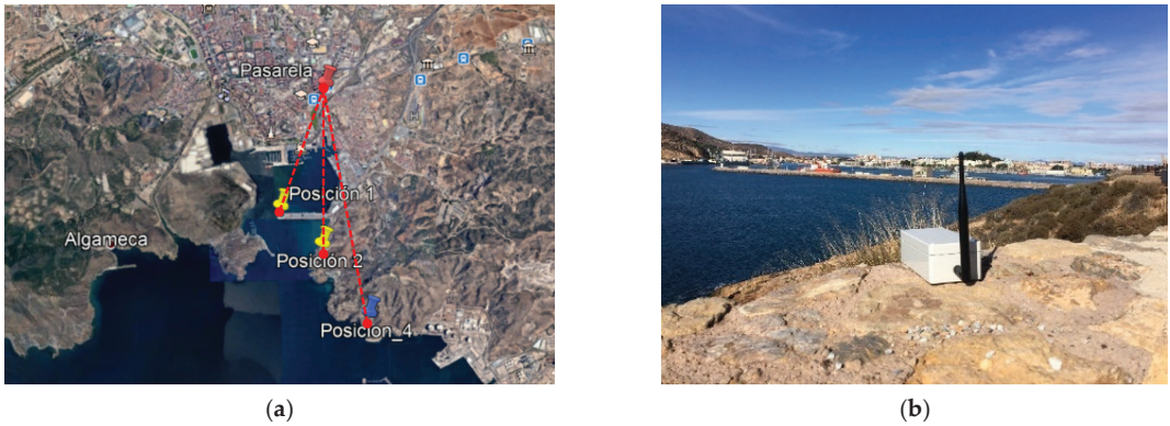
Figure 3. Tested LoRa coverage positions: (a) gateway position and remote points.; (b) photograph of the device at position 2.
