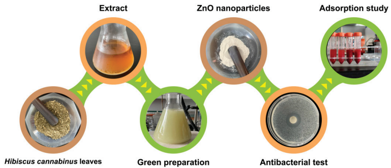
Figure 1. Diagram of the ZnO nanoparticles synthesized using green methods with Hibiscus cannabinus leaf extracts.
