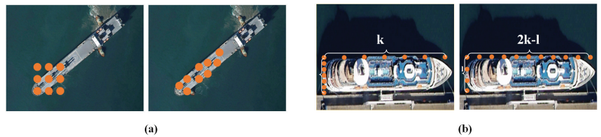
Figure 16. Schematic diagram of methods for large aspect ratios, orange indicates sampling points. (a) Comparison between standard convolution and deformable convolution, and the latter is deformable convolution. (b) Comparison between standard sampling and improved sampling, and the latter better matches the shape.
