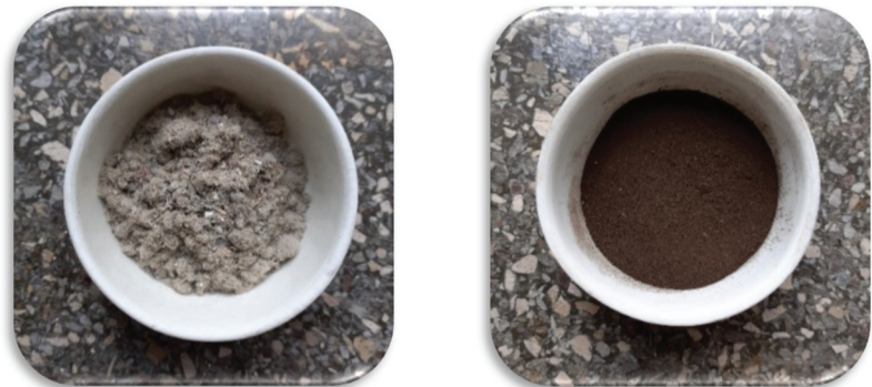
Figure 1. Under-sieve fraction of municipal mixed waste prior to and after hydrothermal carbonization.
