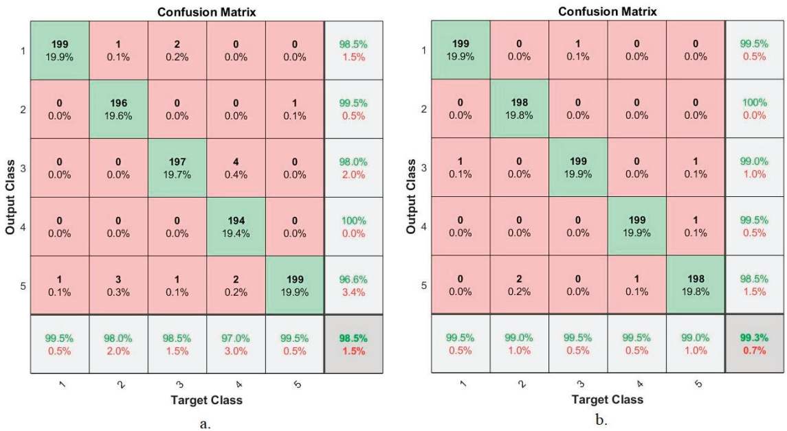
Figure 24. Results of the FFNN for diagnosing lower gastrointestinal diseases based on hybrid features (a) GoogLeNet with traditional algorithm and (b) AlexNet with traditional algorithm.
