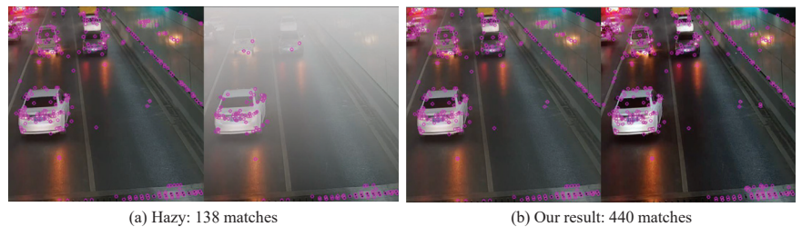
Figure 10. Local keypoints matching by applying the SIFT operator. Compared with the hazy images, the matching results shown that the proposed method can improved the quality of inputs significantly.
