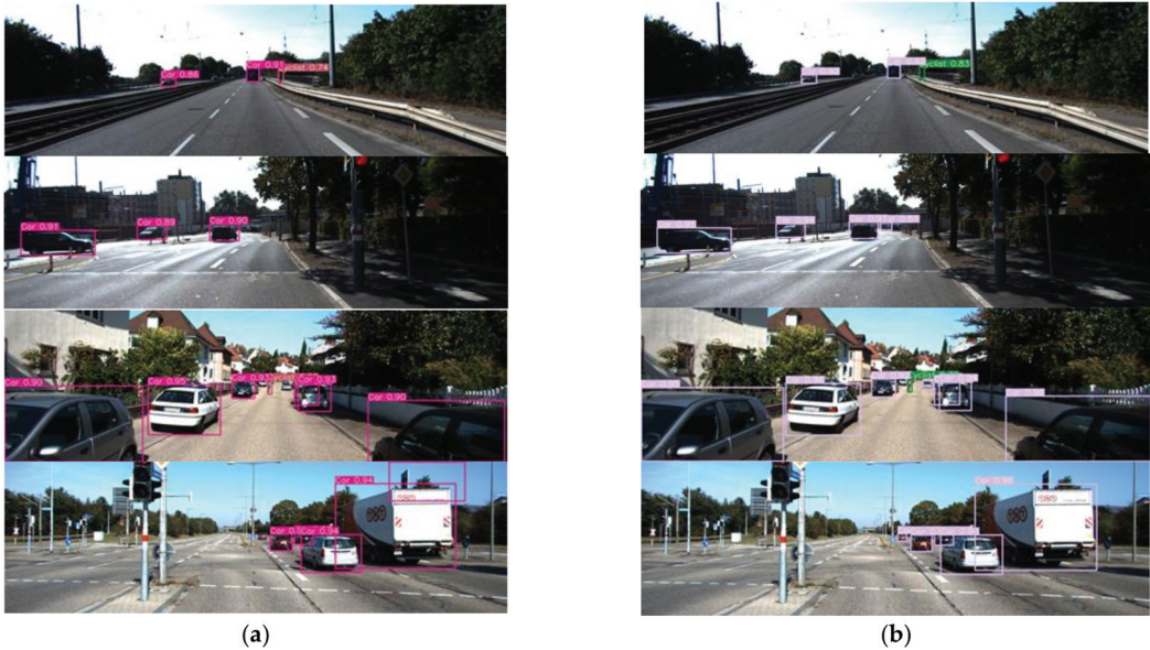
Figure 6. The detection results of YOLOv3 and YOLO-MXANet on the KITTI dataset. (a) YOLOv3. (b) YOLO-MXANet.
