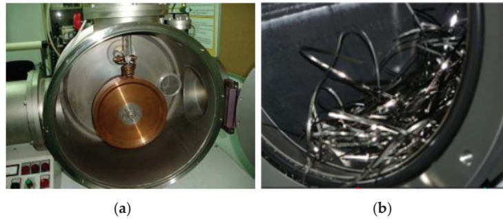
Figure 1. (a) Melt-spun chamber and (b) the obtained as-quenched ribbons.
