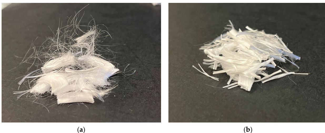
Figure 1. Commercial polypropylene microfibers of similar geometry (both with a length of 12 mm and a diameter of 18 \mu\text{m} ) from different manufacturers: (a) fibers without an additional coating; (b) fibers additionally covered with a water-soluble coating.
