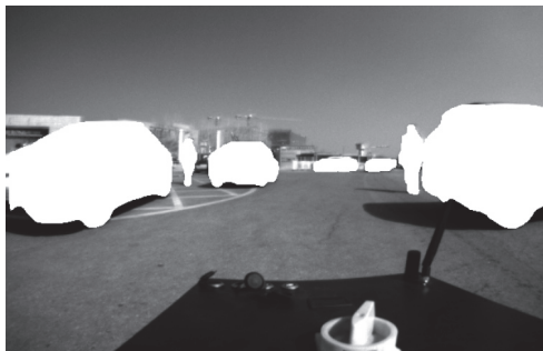
(a) Dynamic target segmentation based on YOLOv7
