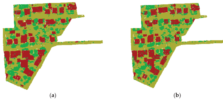
Figure 16. Vaihi-2’s extraction results: ground points are in dark yellow; the facades are in purple; the roofs are in red. (a) Ground truth; (b) the extraction results using the proposed method.
