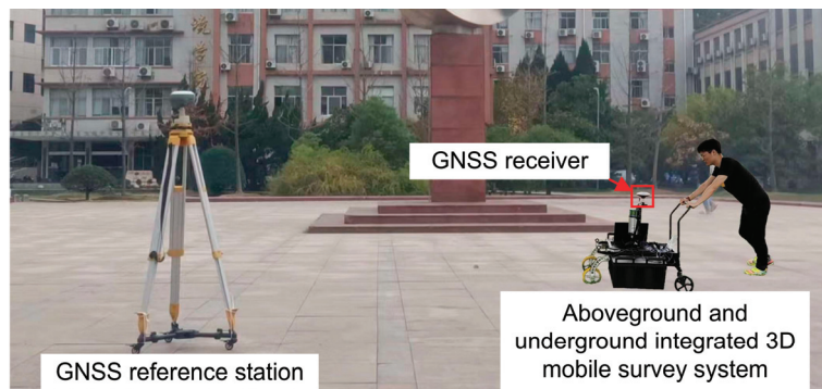
Figure 6. GNSS differential positioning in scene with good GNSS signals.
