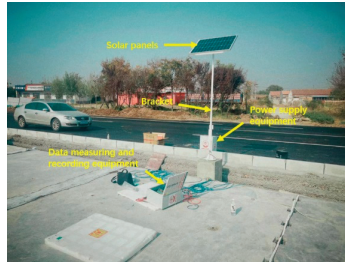
Figure 4. Installation diagram of long-term monitoring equipment.
