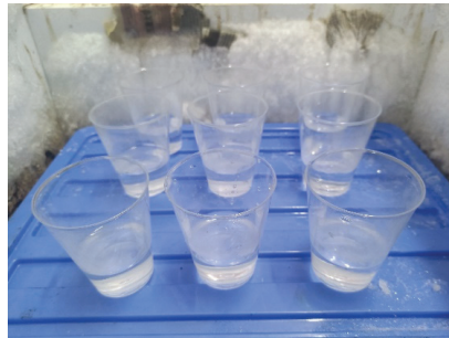
Figure 5. Ice-melting ability test of the solution with gradient concentration.
