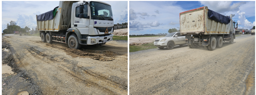
Figure 11. Heavy truck passing on the testbed.
