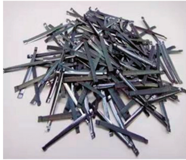
Figure 1. Steel ingot milling profile steel fiber.
