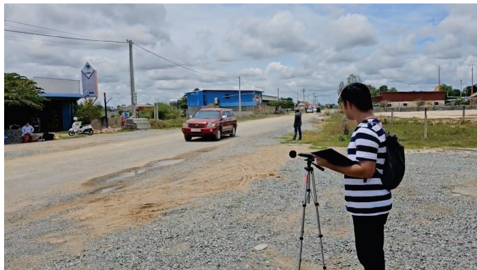
Figure 9. Pass-by test microphone set up.
