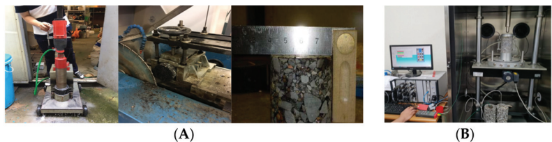
Figure 3. (A) Specimen manufacturing process and (B) Process of measuring dynamic modulus.
