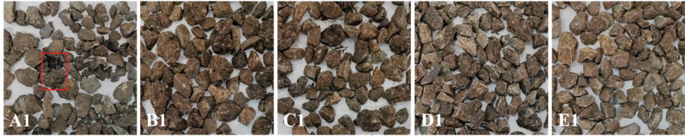
Figure 2. RAP materials with different refined separation frequency parameters. (RAP particles in the red square: false particles; (A1), (B1), (C1), (D1) and (E1) represent 10–20 mm RAP particles after separation at 0 Hz, 30 Hz, 40 Hz, 50 Hz, and 55 Hz, respectively.)
