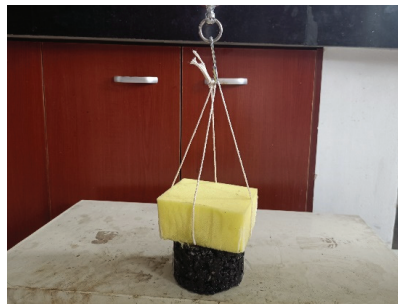
Figure 4. Interface adhesion test.
