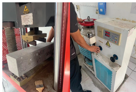
Figure 3. Compression and bending resistance measurement equipment.
