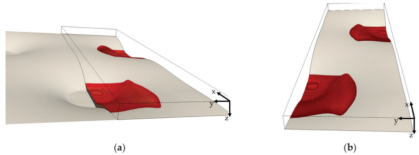
Figure 11. Recirculation zones in the benchmark: side view on the periodic element together with its mirror image (a) and top view (b). Tornado-like vortices upstream the welding spots are shown in dark color. The black lines represent the edges of the computational domain.
