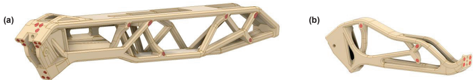
Figure 27. Final CAD model of the 700 mm demonstrator (a) and the 320 mm demonstrator (b). Light red: input and output of the fiber channels into the construction.
