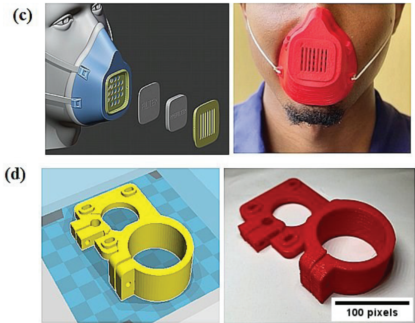
Figure 5. Designed objects printed using the fabricated 3D printing machine: (a) calibration cube; (b) bevel gear, spur gear, outer human ear, and foot; (c) nose mask; (d) fixture holding the electric motor controlling the z-axis.
