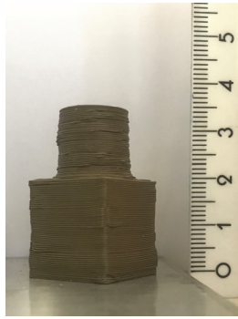
Figure 2. As built part before milling.
