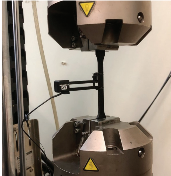
Figure 6. Experimental setup of standard tensile tests.
