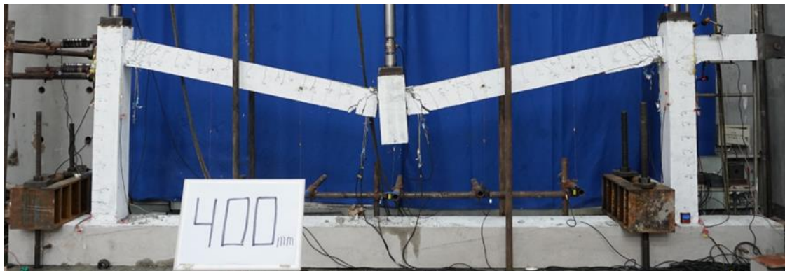
Figure 6. A single-storey reinforced concrete frame under progressive collapse.
