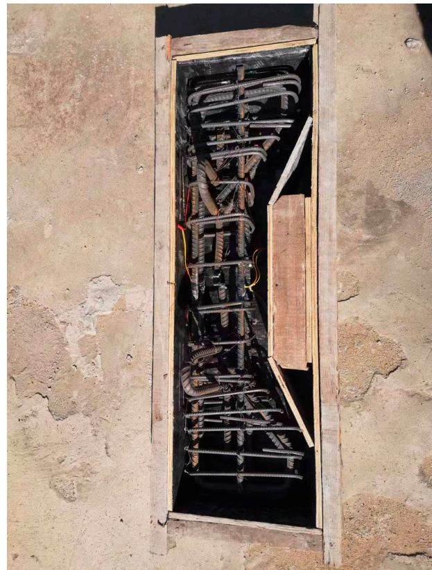
Figure 2. Preparation of specimen: (a) Design of reinforcement (units: mm), (b) Steel bar cage.
