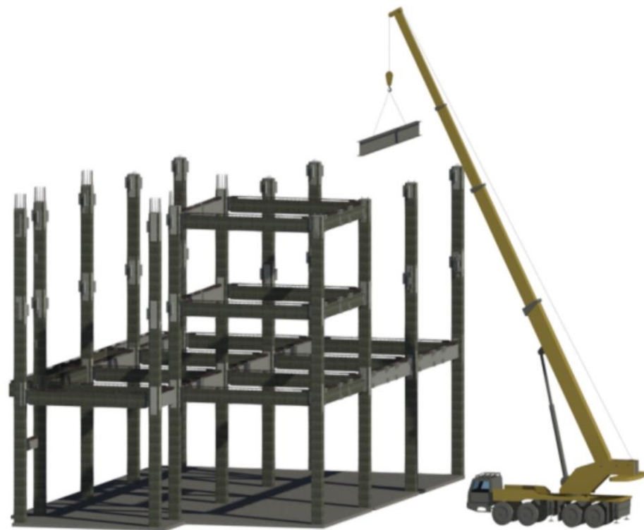
Figure 11. Building construction drawing.
