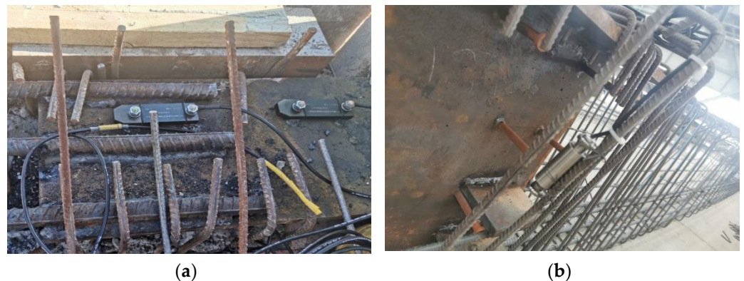
Figure 16. (a) YBM-type tool-type surface strain sensor (b) YNM-type concrete-embedded strain sensor.
