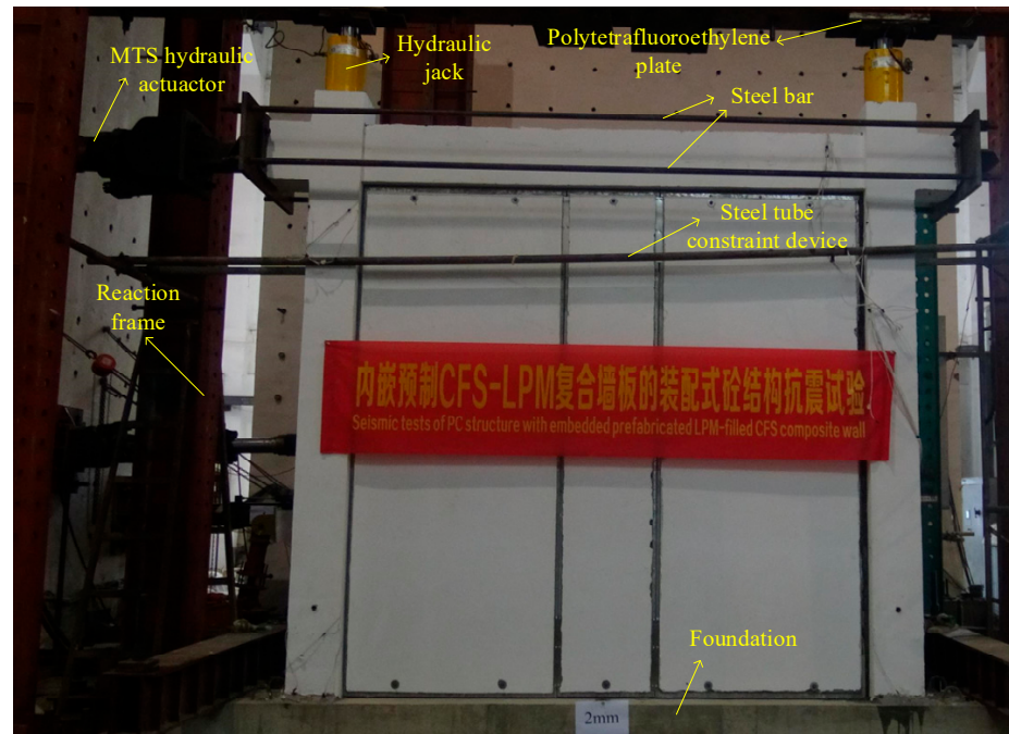
Figure 6. Test set up.
