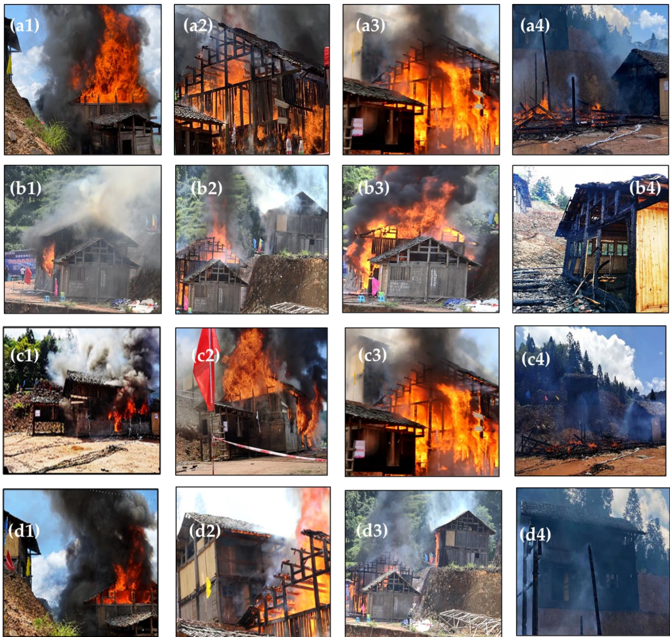
Figure 10. Fire spread among the Houses 1-4 (a,b), of which (a1,b1,c1,d1) were during the time of 10–12 min, (a2,b2,c2,d2) were at the time of 16 min, (a3,b3,c3,d3) were at the time of 19 min, and (a4,b4,c4,d4) were during the time of 23–33 min.
