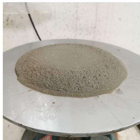
Figure 5. The fluidity test of mortar.
