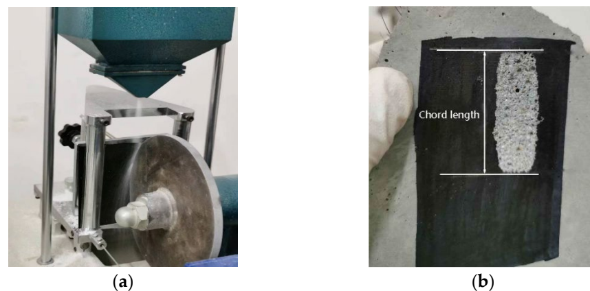
Figure 7. Abrasion resistance tester and tested sample: (a) Abrasion resistance tester; (b) tested sample.
