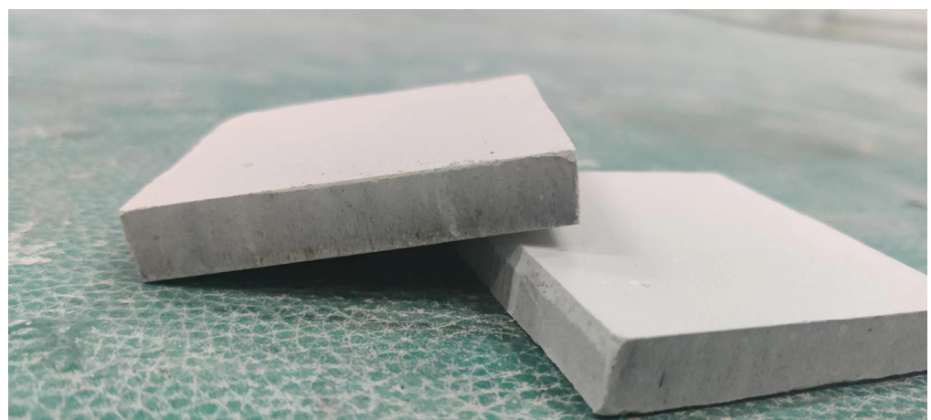
Figure 3. A 60 \text{ mm} \times 60 \text{ mm} \times 10 \text{ mm} rectangular specimen schematic diagram for raw meal.
