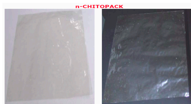
Figure 14. CS/CN film produced by the casting technique.
