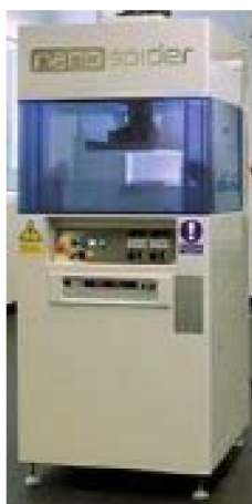
Figure 1. The used electrospinning setup.
