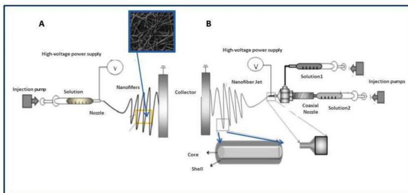
**Figure 3.** Schematic diagram of electrospinning setup consisting of injection pump/s, power supply, nozzle and conducting collector. A: One type of solution. B: Two type of solution and a core-shell nozzle design used to encapsulate drugs within the nanofiber. Adapted from Shin, S.H. et al. [24].
