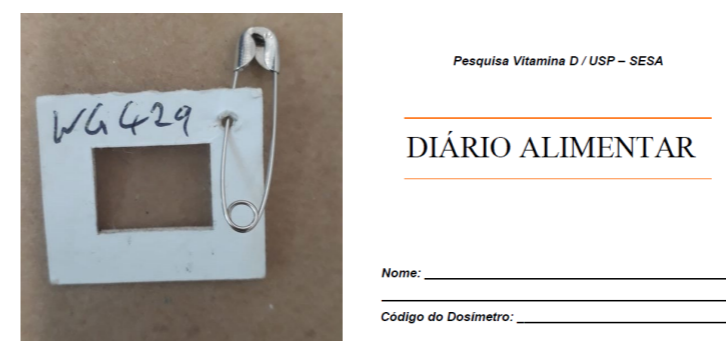
Figure 4. On the left a polysulphone badge and sheet and on the right a food diary.
