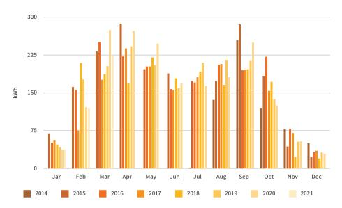
**Figure 4.** Monthly renewable energy generation of the façade PV system since installation in 2014. Source: Graphic by author.
