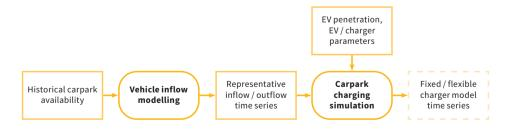
Figure 7. Workflow for EV charger demand modeling. Source: Graphic by authors.
