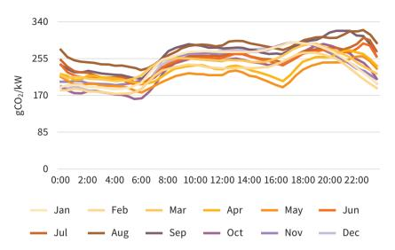
**Figure 3.** Monthly averaged UK grid electricity carbon intensity 2020 (half-hourly data). Source: Graphic by author.
