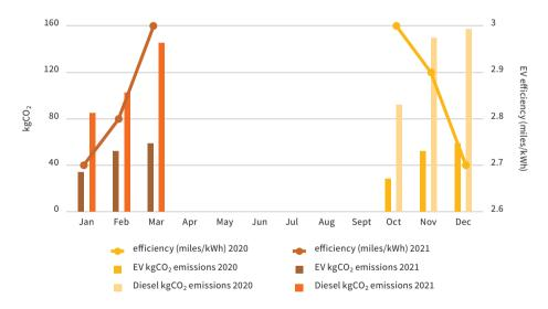
**Figure 8.** Carbon emission comparison between electric vehicle and diesel vehicle, plus electric vehicle efficiency. Source: Graphic by author.
