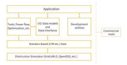
**Figure 2.** Overview of the software architecture of GridAPPS-D. Source: Graphic by authors, information adapted from (Melton et al. 2019).
