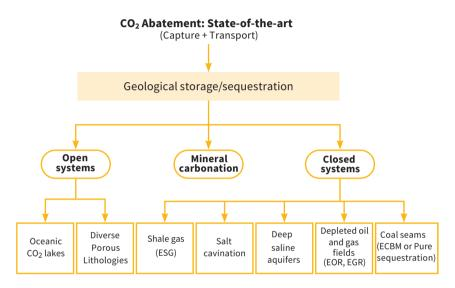
**Figure 16.** Geological storage solutions for CO<sub>2</sub> abatement. Source: Graphic by authors, adapted from Lemos de Sousa et al. (2008).
