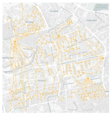
**Figure 5.** Synthetic grid layout for the Geylang District in Singapore. Source: Graphic by authors.
