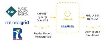
**Figure 3.** Power distribution network model conversion workflow via CIMHub. Source: Graphic by authors.
