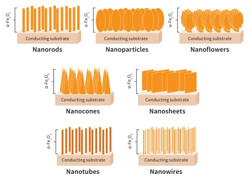
**Figure 5.** Schematic illustration of different morphologies of hematite films for PEC water splitting. Source: Graphic by authors.
