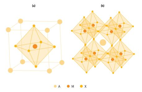
**Figure 1.** Cubic crystal structure (**a**) and A-Cation in 12-fold coordinated voids of the  $MX_6$  octahedral inorganic framework (**b**) of HaP with general formula  $AMX_3$ . Source: Liu et al. (2015b).
