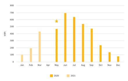
**Figure 5.** Monthly renewable energy generation of the roof PV system since installation in May 2020. NB: The star highlights that May 2020 data only represents 15 days. Source: Graphic by author.
