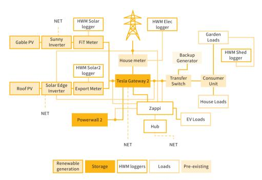
**Figure 2.** Schematic of equipment for monitoring renewable generation and storage. Source: Graphic by author.
