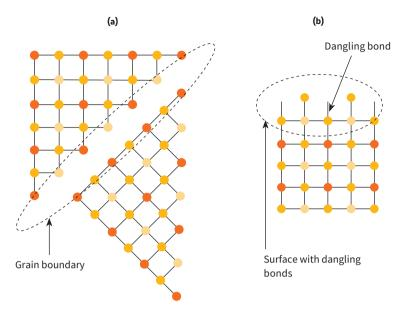
**Figure 2.** Schematic diagram showing grain boundaries (**a**) and surface defects (dangling bonds) (**b**) in HaP. Source: Graphic by authors.
