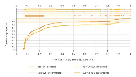
**Figure 11.** Substation transformer utilization for uncontrolled charging. Source: Graphic by authors.
