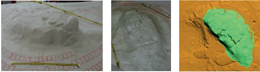
Figure 5. The historic physical 3D model of the Kalkberg (left), the historic digital 3D model from dense image matching (centre) and the combination of two DEMs from both today (orange) and the past (green) (right).
