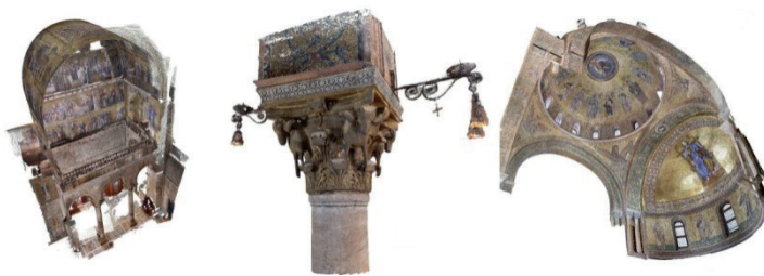
Figure 2. Images of two models at different resolutions, according to the needs of modelling and orthophoto. From the left: model of the whole area with 35 mm, model of a capital with 85 mm, model of the dome with 200 mm for orthophoto.
