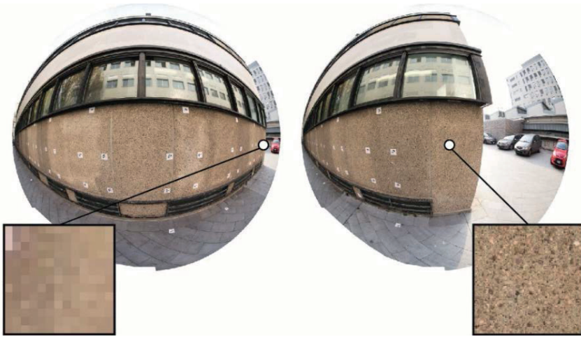
Figure 1. Two circular fisheye images of a straight wall; the same area was rendered at a very different resolution when placed in the centre or on the border of the frame.
