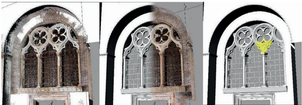
Figure 5. Example of modelling of a complex architectural element (gothic window) from a point-cloud to a non-uniform rational B-spline (NURBS) model.
