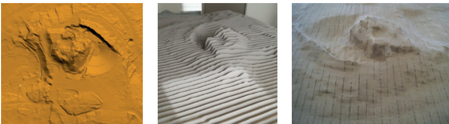
Figure 4. The reconstruction of the Kalkberg from airborne laser scanning data: digital elevation model (original data, left), printed scaled sections of the DEM (centre) and physical 3D model of today's existing Kalkberg (right). Photos centre and right: Nils Hinrichsen.
