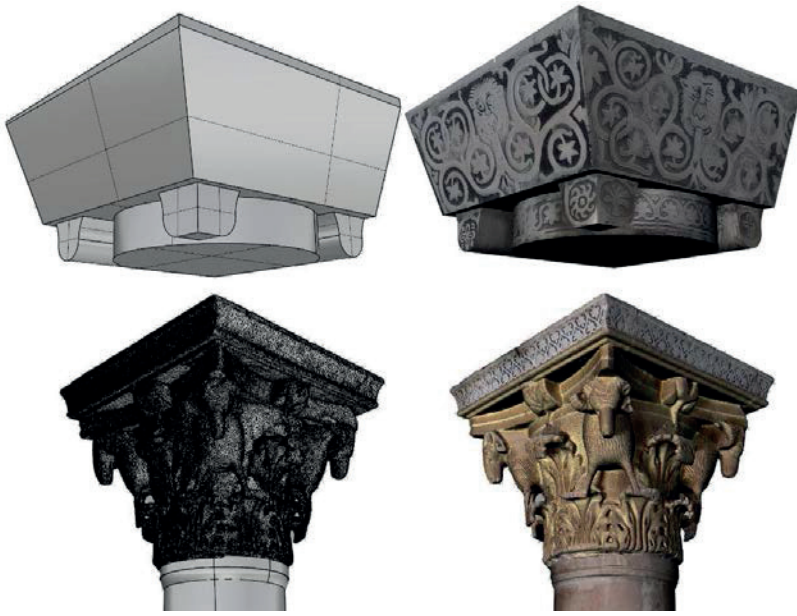
Figure 7. Two capitals modelled in different ways according to their complexity. Above, a simpler capital modelled with NURBS, below the complex one, modelled with mesh.
