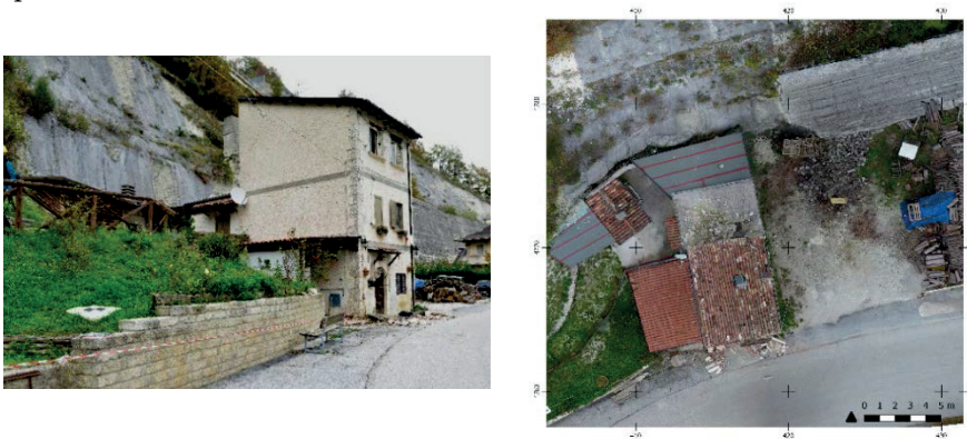
Figure 14. An images of the building n°5 in October 2016 and relative orthoimage by multi-rotor drone (aerial images of both shooting and frames extraction from 4k video with DJI drone).
