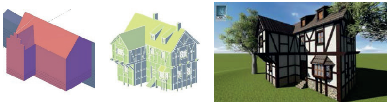
Figure 9. Development of a building in the outer ward: Initial CAD model (left), detailed model (centre), textured model in Lumion 3D (right).
