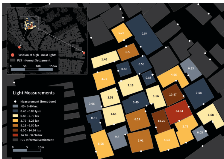
Figure 8. Lux measurements taken at each household's front door, where less than 1 lux (blue) is below the City of Cape Town's accepted standards. Source: Reprinted from (Briers 2023), used with permission.
