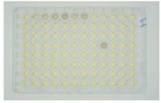
Figure 3.7. Microtiter plate after completion of the assay. A yellow colour indicates a low-, a brown colour a high-phenylalanine concentration in the original blood sample.
