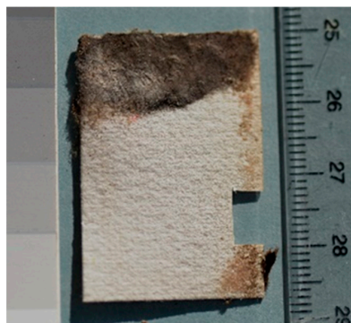
(c) W&N paper, recto, fungi was cultured in darkness. The dark colony along the top was a contamination and not the inoculant. Inoculant was applied along the vertical, longer edge and showed meager growth.
