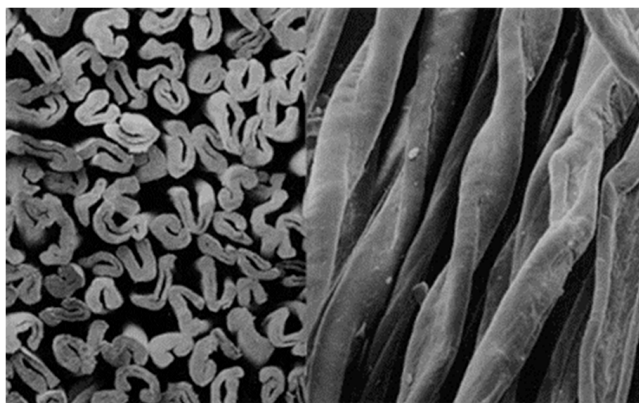
Figure 2.16. Longitudinal study and cross-sections of cotton fibers. The characteristic, ribbon-like twist is one of the identifying features of cotton fibers. The cross-section of cotton fibers shows the water entry areas. SEM micrograph. Source: Reprinted from http://www.freewebs.com/textile-technology/fibrescience.htm (accessed on 13 April 2012).
