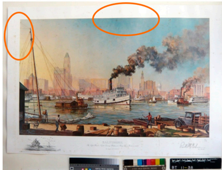
Figure 3.1. A commercial chromolithograph shows foxing stains scattered around the edges; details are shown in Figures 3.2–3.5. Artwork by P. McGehee, Baltimore , 18 3/4" × 30". The areas with high concentrations of stains are indicated by oval demarcations. Source: Figure by author.
