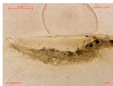
Figure 1.9. Bio-deposits in the paper matrix are shown on a cross-section of paper with stains; black fungal cells are near the surface and just below the surface. A sample of the 1920 Engraving, Study Case No. 3, embedded in resin was examined using transmitted light microscopy followed by observations in SEM-VP. Transmitted light micrograph of a cross-section of a fungal stain on paper shows the extent of microbial penetration; scale 50 µm. Source: Figure by author.
