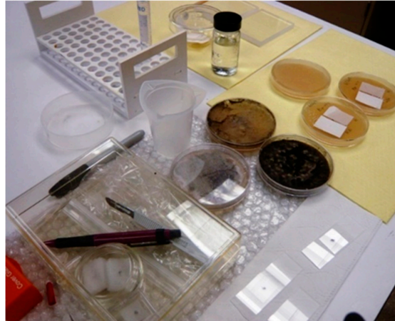
Figure 2.28. The setup of the bio-simulation experiment: Petri dishes, inoculating needle, pure inoculant Aspergillus niger , and sterilized model papers (Whatman 4 and Winsor & Newton). Source: Figure by author.
