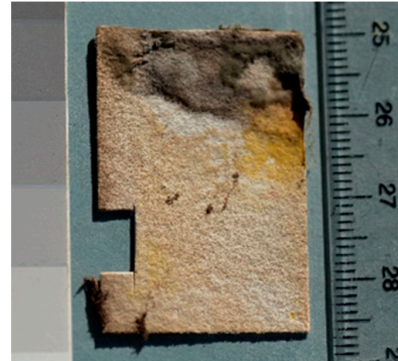
(d) W&N paper, reverse side of sample on which fungi grew in darkness.
