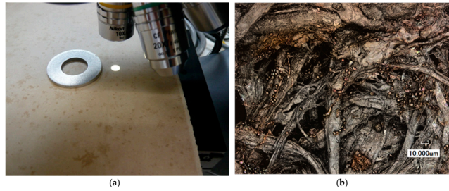
Figure 5.3. (a) An artwork with foxing stains is examined using a scanning laser microscope. This microscope permits carrying out the examination without removing samples from the original material. The metal ring shown here was used as a weight to ensure an even scan of an undulated paper; its use is optional. (b) An example of an image produced by confocal scanning laser microscopy. Paper fibers are covered by fungal conidia. Instrument used: Keyence, 3D Laser Scanning Microscope, VK-9700. Scale 10 \mu\text{m} . Source: Figure by author.
