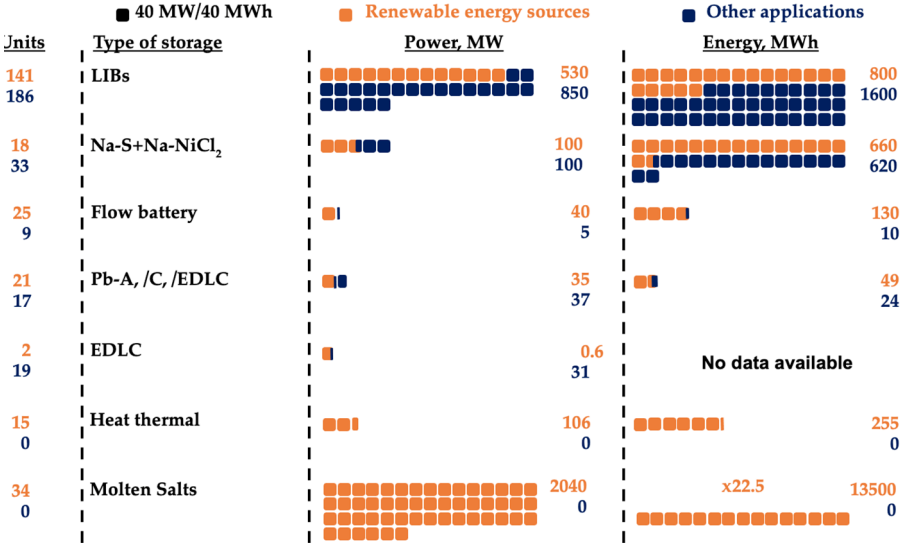
Figure 57. Installed energy and power capacity of stationary electrochemical and thermal energy storage used in the generation of energy from renewable sources [1]. Source: Figure by authors.
