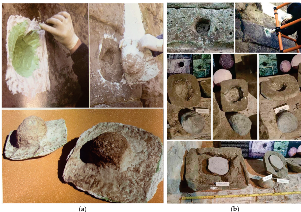
Figure 3. (a) Pompeii, silicone mold 2002. (b) Above left: a trace from a ballistic impact; above right, technicians at work. Below, the negative molds and positive casts currently preserved at the Saepinum area, Altilia, CB. Images courtesy of F. Russo private archive.
