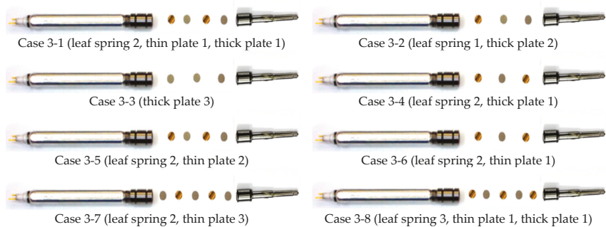
Figure 11. Detailed designs of Type 3 DPIs.
