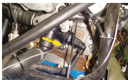
Figure 7. View of the combustion pressure sensor installed in the fired cylinder of the research engine (location of the sensor is indicated by the yellow arrow).
