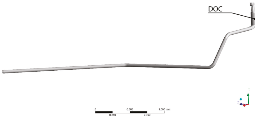
Figure 6. Three-dimensional geometry model of the exhaust system.
