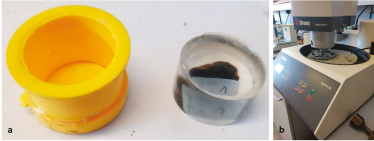
Figure 3. Plastic mold for preparation of the stone-resin samples (a) and the polishing machine (b).
