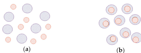
Figure 1. Differences between mixture of two aqueous dispersions of different polymers (polymer 1—blue color and polymer 2—red color) and aqueous dispersion with hybrid particle structure composed of the same two different polymers. In the mixture of two dispersions (a) synergistic effect is much less probable than in dispersion with hybrid particle structure (b) [4].
