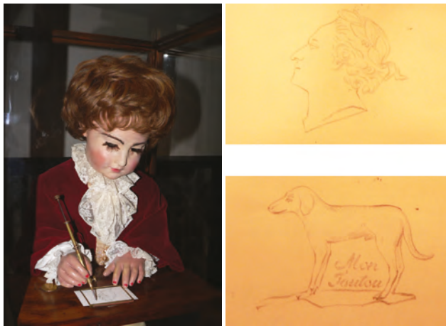
Figure 1. The “Artist” painting automaton by Jaquet-Droz ( Left , Rama (2005) ) along with two of the four images that it can draw: a portrait of Louis XV ( Top Right ) and a drawing of a dog with “Mon toutou” written next to it ( Bottom Right ) Droz (ca. 1770) .
