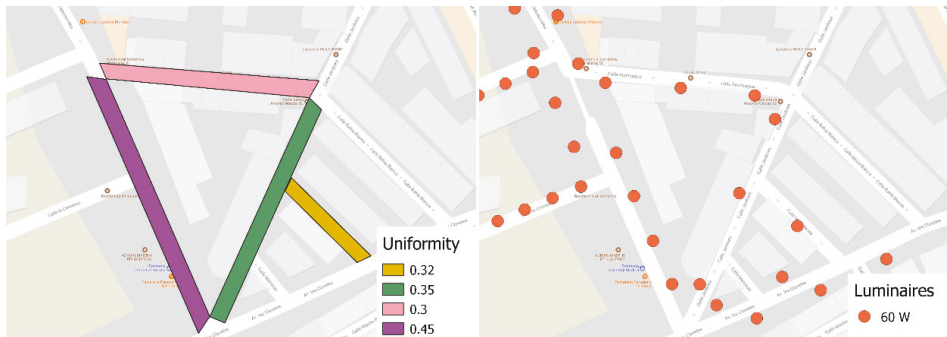
Figure 14. Illuminance uniformity (left) and luminaires position (right).
