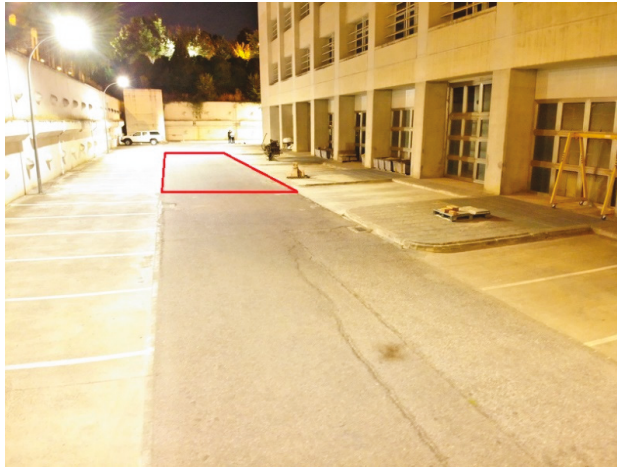
Figure 5. Digital image in which the calculation area of average luminance is indicated by a red frame. According to the standard procedure the camera is located at a distance of 60 m from the calculation area and at a height of 1.5 m.
