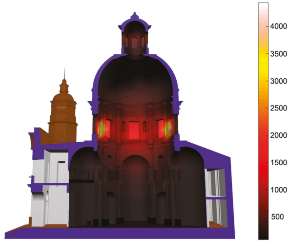
Figure 21. Daylight Section at the spring equinox in a cloudy situation. Maximum values of 200 lux on the ground. Source: Cabeza-Lainez and Almodovar-Melendo.
